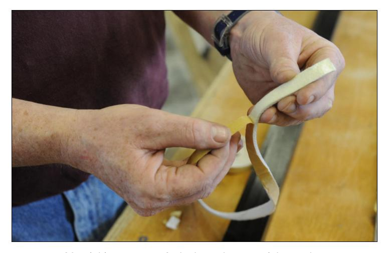
WNG uses self sticking contact cloth where the tray picks up the underlever. The first step is to peel back the backing paper.
