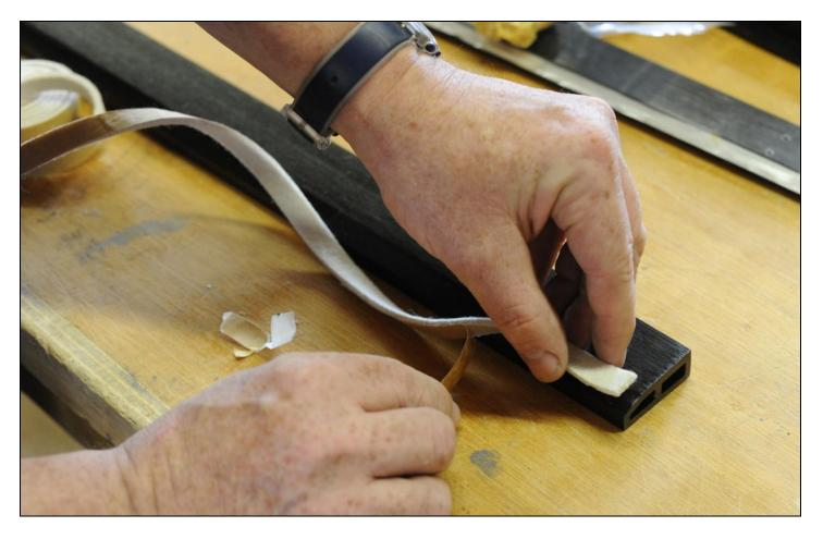
Install the contact cloth in the defined place on the tray so that is against the inner edge.
